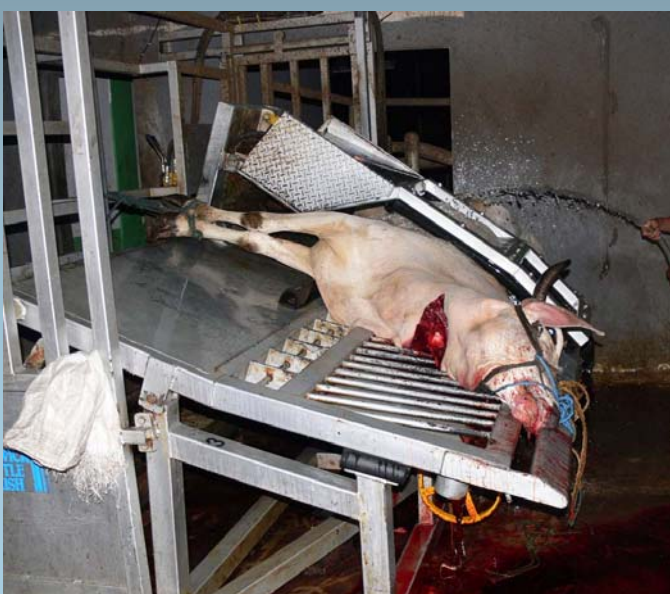
Figure 2 Mark 4 restraint box with local Indonesian animal
